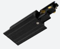
Einspeiser, DALI, Erde links 16A max. | Polycarbonat (PC) L: 14.7 cm | B: 5.6 cm | H: 3.3 cm
